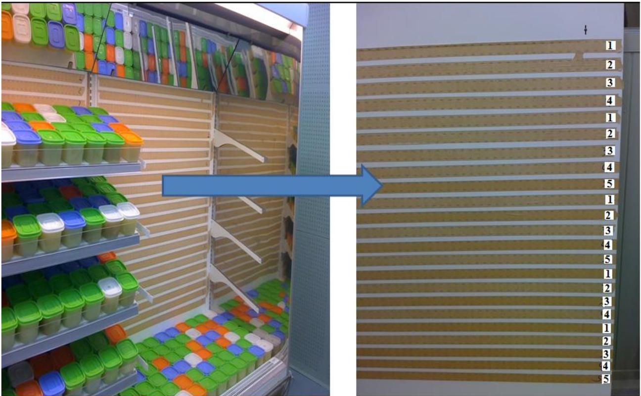
Figure 3. Open refrigerated display cabinet with perforated back panel completely closed.
